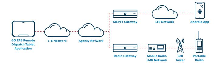
In a typical configuration from a remote dispatch location or work-from-home environment, GO TAB connects to your organization's IP Network through a Wi-Fi Internet or LTE network connection with Cradlepoint Routers.
